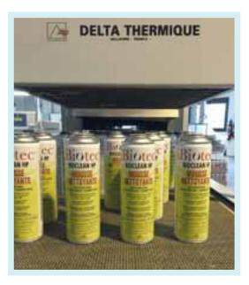
The team at iBiotec implements quality on-site printing of graphics and decoration onto containers using screen-printing or pad printing methods. Equipped with 9 printing lines, iBiotec can print up to 4,000,000 units.
