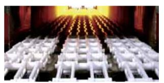
Industrial oven chain conveyor lubrication. Continuous firing of phenolic/silver conductive polymers at 428 °F
