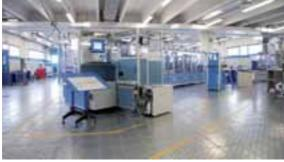
Cleaning and degreasing assembly line stations.
