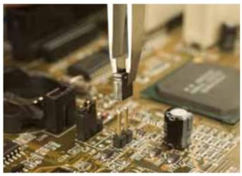
Cleaning of micro-electronic contacts and electronic circuits.
