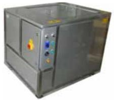
Degreasing, cleaning and washing mechanical components in ultrasonic cleaning with piezoelectric or magnetostrictive transducers.
