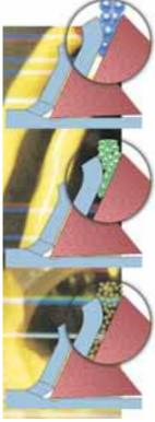
Crowding of emulsion molecules at tool-swarf interface prevents correct penetration.
